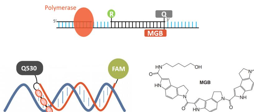
**Figure 4.** Principle design of MGB probes. Incorporating a minor groove binder (MGB) stabilizes the probe-target duplex and increases the melting temperature ( $T_m$ ), enabling the use of shorter probes. The chemical structure is shown (bottom right), along with a schematic representation of probe hybridization with the target (bottom left)..
