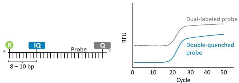
**Figure 2.** Design and qPCR performance of double-quenched probes. The additional quencher placed 8–10 bp from the 5' reporter (left) enhances energy transfer, making these probes ideal for longer designs. This results in reduced background fluorescence compared to dual-labeled probes, as demonstrated in qPCR using a 30 nt probe (right, no baseline subtraction applied).
